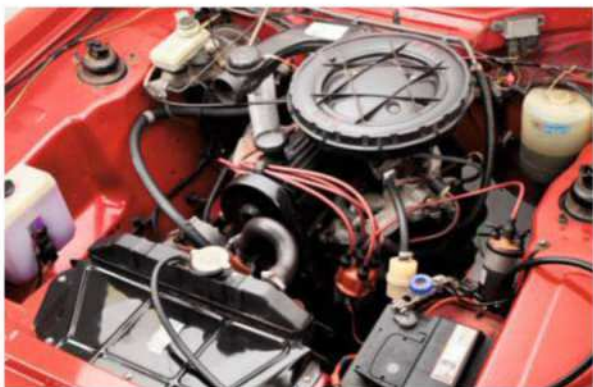
This is the 1.6 engine, but all the Capri power units are strong and simple to work on, mostly with good parts availability
