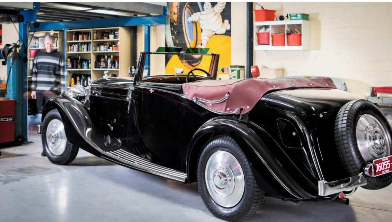
Spare wheel had to be relocated from the nearside running board to its correct home at the rear
